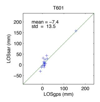
Comparisons of vector deformation from ALOS interferometry with highly accurate 3 GPS vector displacements derived from continuous measurements surrounding Kilauea (red triangles previous figures). LOS errors are typically 14 mm rms while the displacement derived from pixel matching has an rms error of 70 mm.
