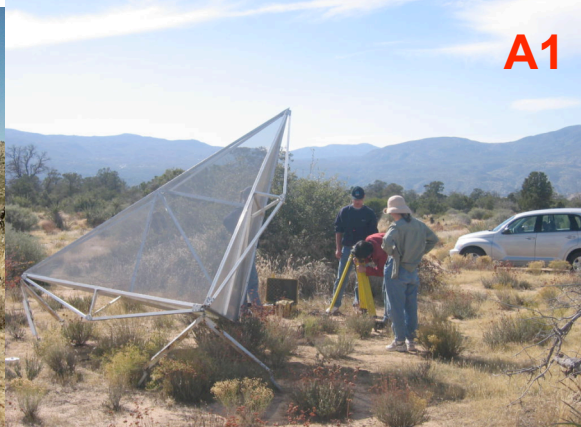
Figure 3. Photographs of the 3 radar reflectors. Reflectors D1 and D2 were installed at Pinon in 1997 were originally oriented to reflect radar from ERS-1 and ERS-2 having incidence angles of 23^\circ and azimuth of 102.5^\circ . In July of 2004 the reflectors D1 and D2 were adjusted to optimally reflect ALOS data with incidence angles between 34^\circ and 43^\circ . In November of 2005 the ascending reflector was installed to reflect radar waves having an azimuth of 257.5^\circ to reflect ALOS data along ascending passes.
