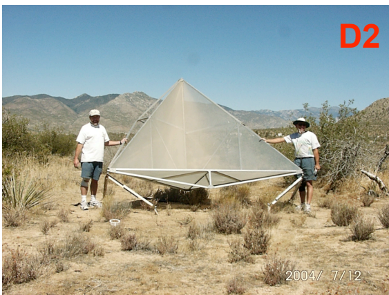
Figure 3. Photographs of the 3 radar reflectors. Reflectors D1 and D2 were installed at Pinon in 1997 were originally oriented to reflect radar from ERS-1 and ERS-2 having incidence angles of 23^\circ and azimuth of 102.5^\circ . In July of 2004 the reflectors D1 and D2 were adjusted to optimally reflect ALOS data with incidence angles between 34^\circ and 43^\circ . In November of 2005 the ascending reflector was installed to reflect radar waves having an azimuth of 257.5^\circ to reflect ALOS data along ascending passes.
